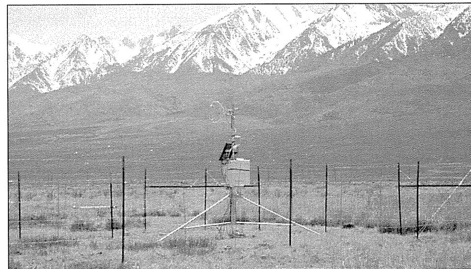
Meteorological instruments used to measure evapotranspiration from an alkali meadow. Photo by Bob Harrington, ICWD.
