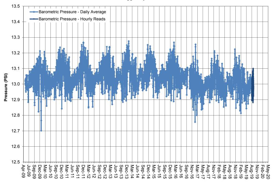
Note: BaroTroll located in well casing of well HR-2B. Used to adjust pressure readings in non-vented transducers. BaroTroll stopped working and was replaced 10/19/2016.
