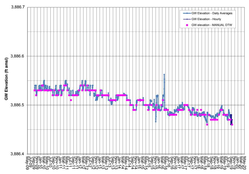
Note: Vented transducer data correlated to Manual DTW measurements. DTW measured to .01 foot; GWE calculated using approximate surface elevation. Coso Operating Co. initiated Hay Ranch Project pumping on 12/25/09.
