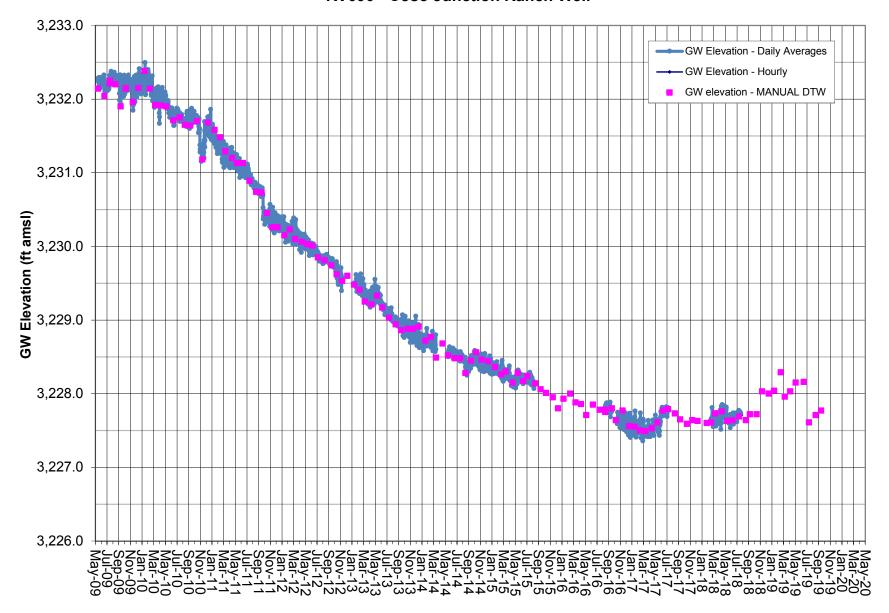
Note: Transducer data (absolute pressure) adjusted by data logged from BaroTroll and correlated to Manual DTW measurements. COC initiated Hay Ranch Project pumping on 12/25/09.
