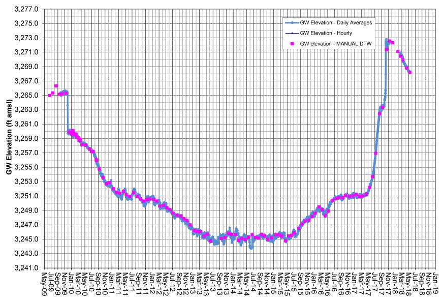
Note: Transducer data adjusted by BaroTroll and correlated to Manual DTW.
