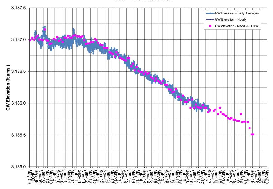
Note: Transducer data (absolute pressure) adjusted by data logged from BaroTroll and correlated to Manual DTW measurements. Well damaged and transducer missing on Oct. 2017.
