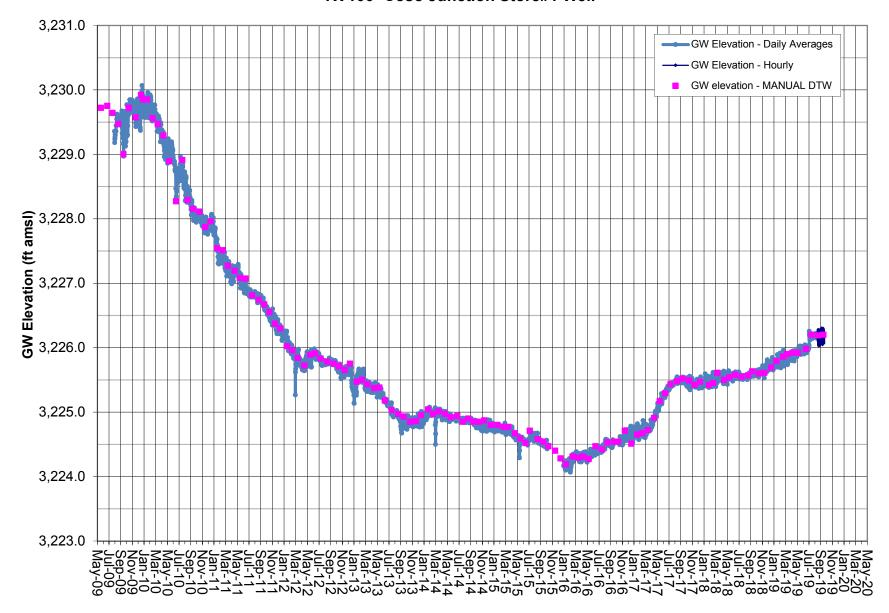
Note: Transducer data adjusted by data logged from BaroTroll and correlated to Manual DTW. Data gap from Oct.-Dec. due to pressure transducer malfunction.
