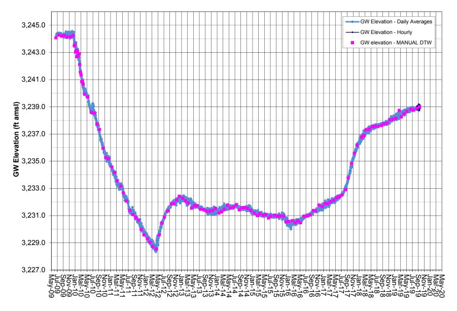
Note: Screened interval 170-260 feet. Coso Operating Co. initiated Hay Ranch Project pumping on 12/25/09. HR 1A data gaps due to transducer malfunction.
