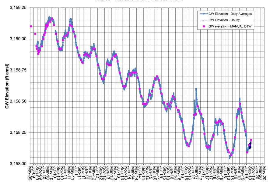
Note: Vented transducer data correlated to Manual DTW measurements. Coso Operating Co. initiated Hay Ranch Project pumping on 12/25/09. Transducer replaced on 9/20/18.
