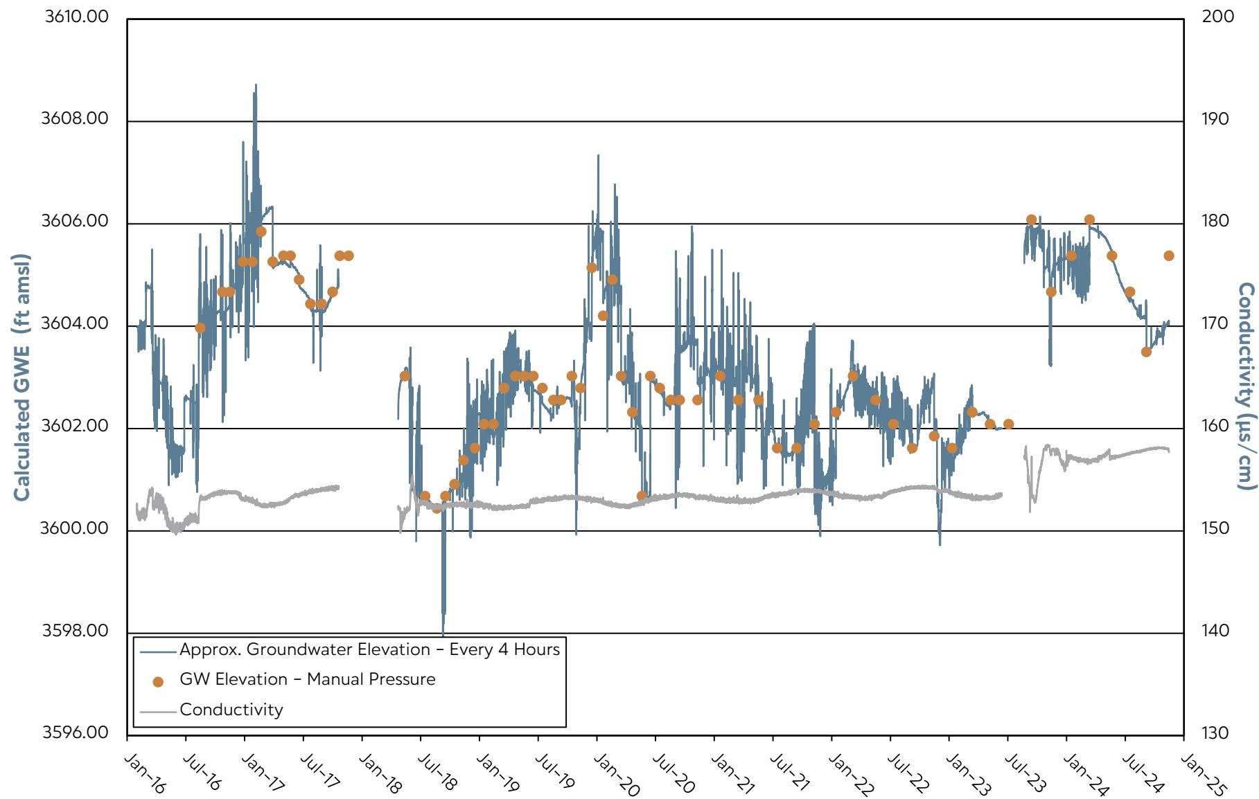
Note: Artesian Well. Transducer data from AquaTroll200 correlated to manual pressure and converted to GWE.
