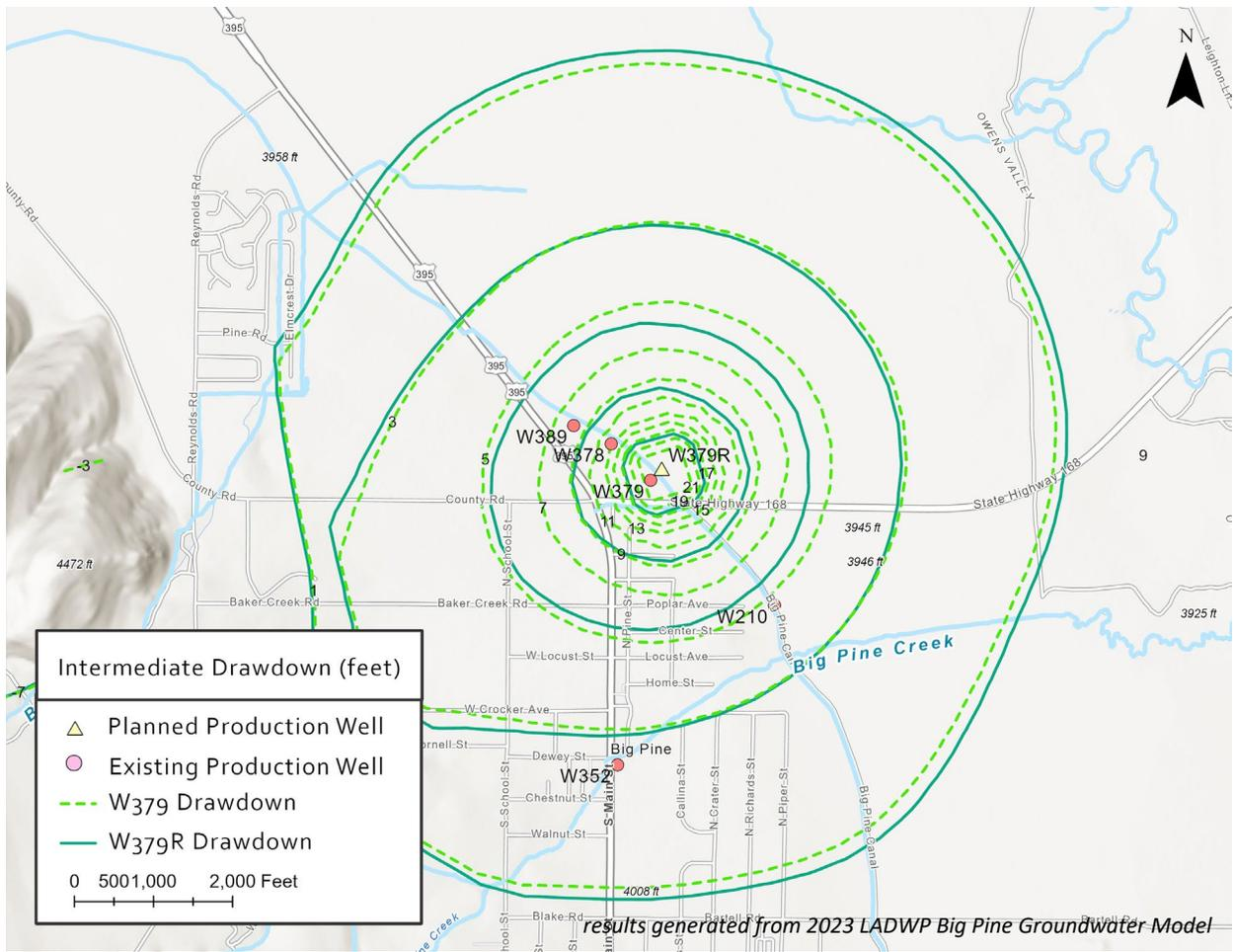
**FIGURE 9 - INTERMEDIATE AQUIFER GROUNDWATER DRAWDOWN (FT) FROM OPERATING EXISTING W379 AND REPLACEMENT W379R AT 4.3 CFS FOR ONE YEAR**
