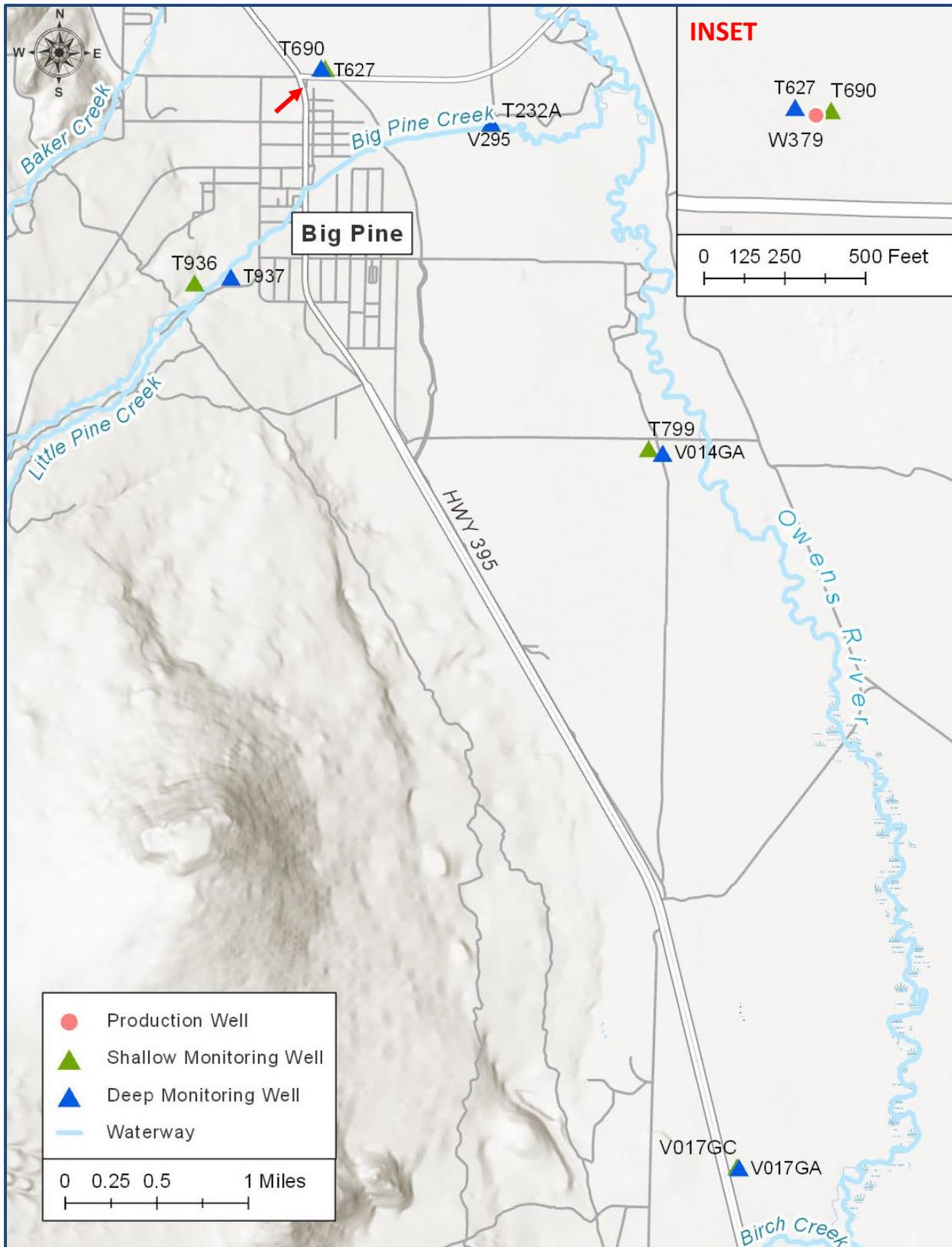
**FIGURE 2 – SHALLOW AND DEEP AQUIFER MONITORING WELLS IN BIG PINE WELLFIELD**
