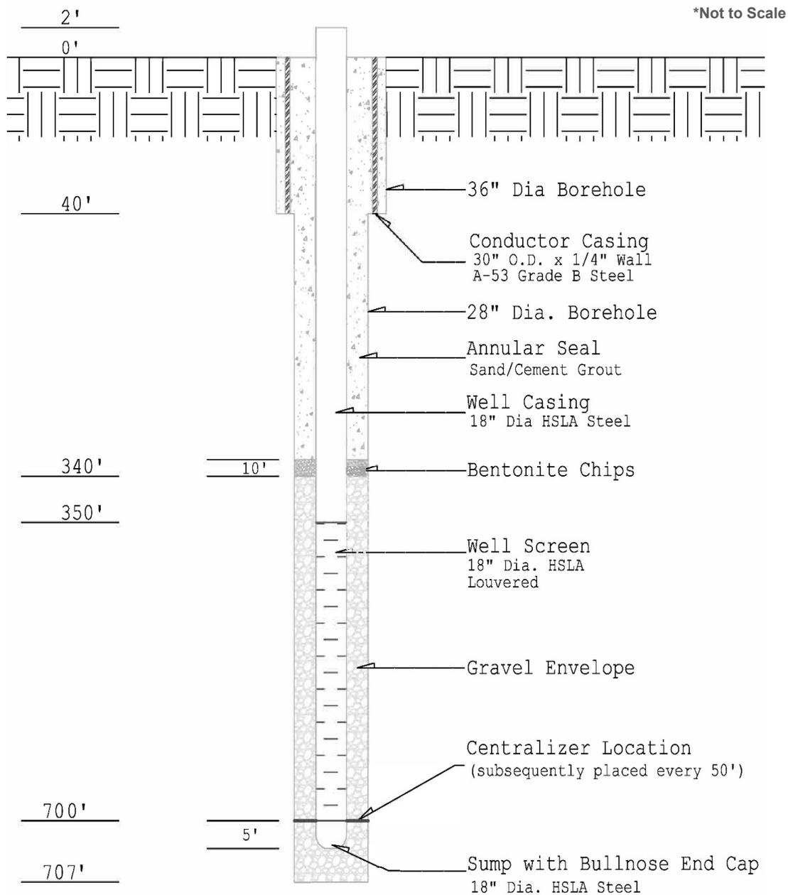
**FIGURE 7 - PRELIMINARY DESIGN FOR W379R IN BIG PINE WELLFIELD**
