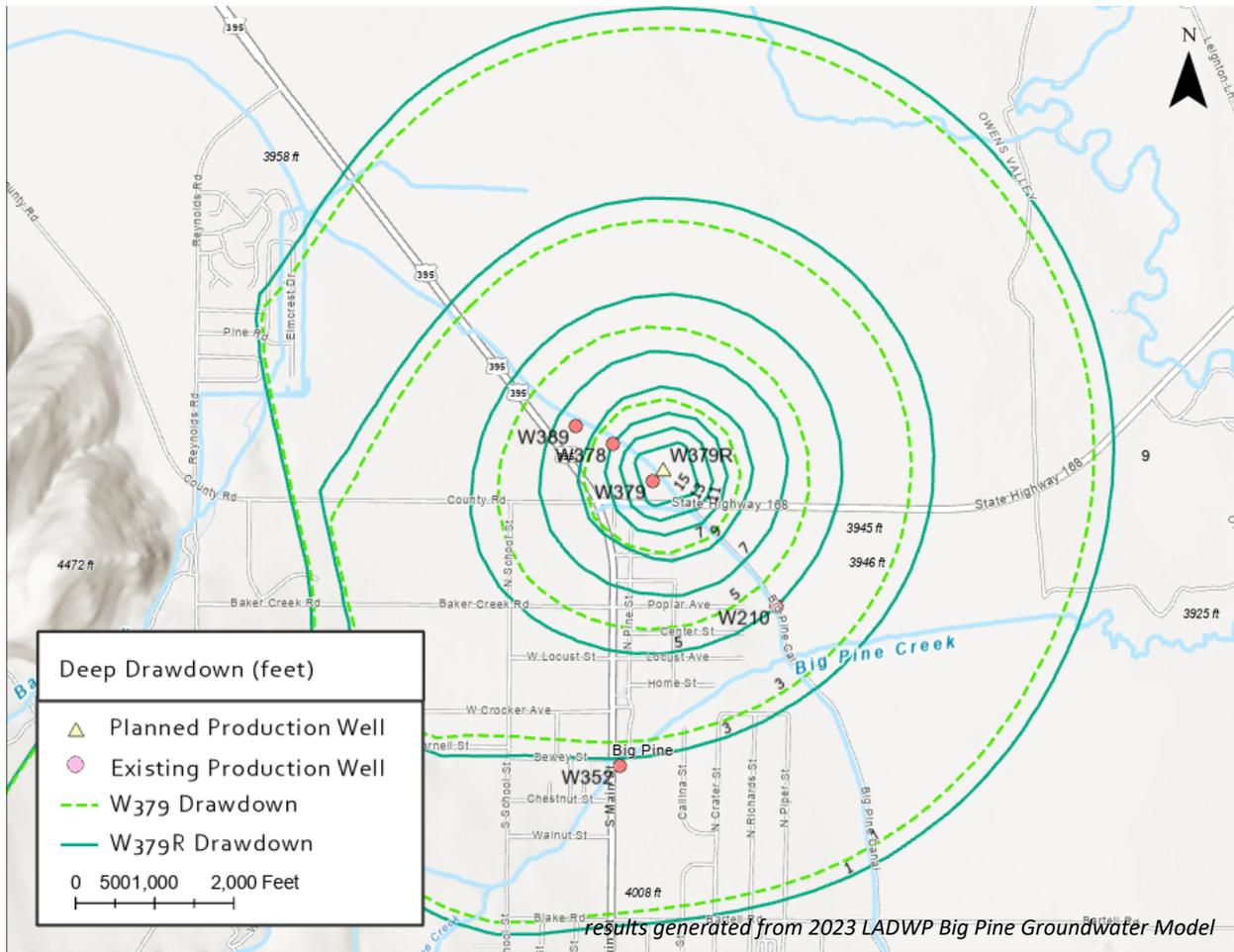
**FIGURE 10 - DEEP AQUIFER GROUNDWATER DRAWDOWN (FT) FROM OPERATING EXISTING W379 AND REPLACEMENT W379R AT 4.3 CFS FOR ONE YEAR**
