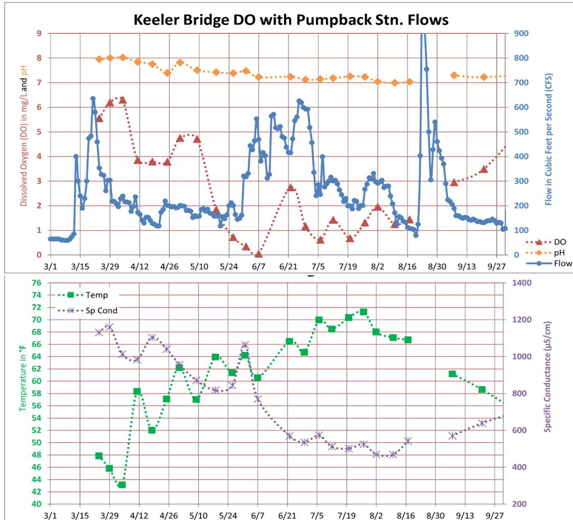
**Figure 3-6. 2023 LOR Flow with DO and pH at Keeler Bridge. Minimum DO coincides with initial summer peaking of flow (June 7). Flow data are taken from the Pumpback Station discharge gauging station. Gaps in water quality parameters indicate measurements missed due to site inaccessibility.**
