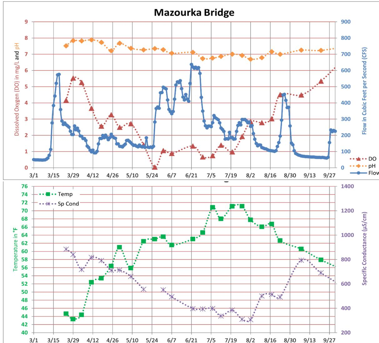
Figure 3-4. 2023 LOR Mazourka Bridge. LOR Flow with DO, pH, Temp, and Sp Cond at Mazourka Bridge.
