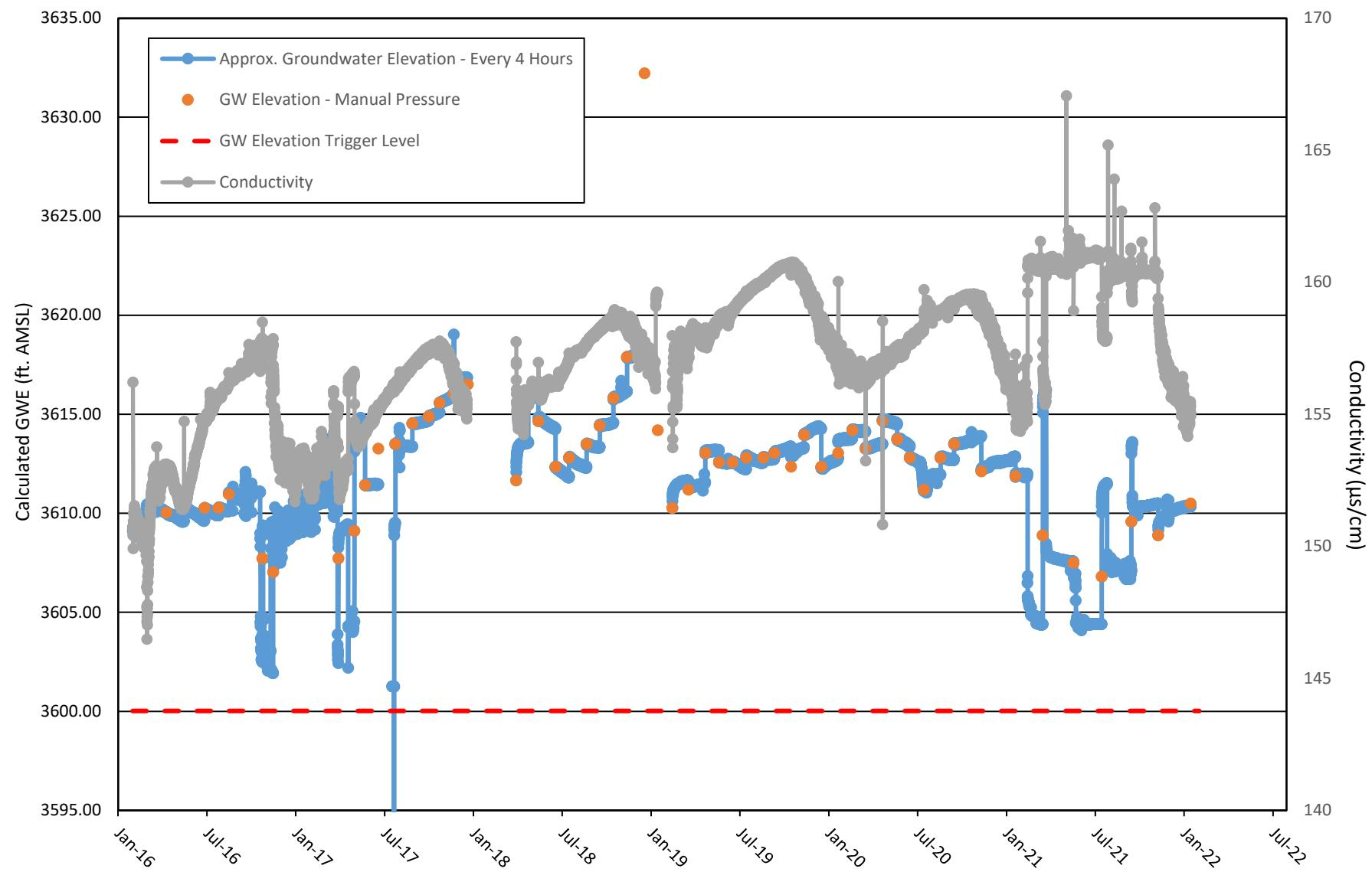
Note: Artesian Well. Transducer data from AquaTroll 200 correlated to reference pressure and converted to GWE.
