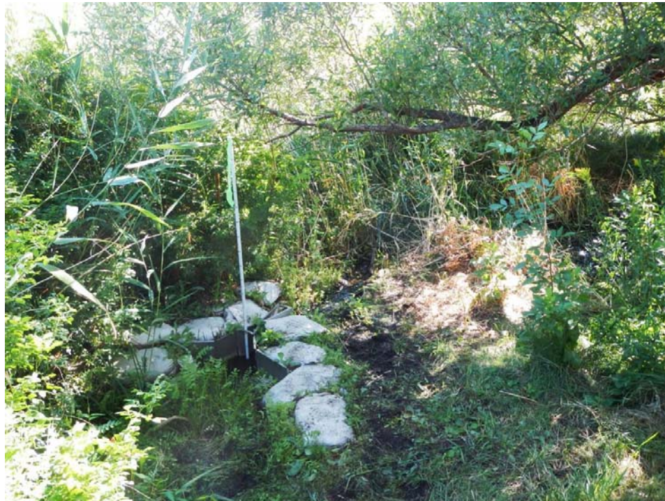
Photo 4: CBS 2 – The spring originates underneath dense common reed just to the right of the flume (surrounded by cement bags) in the center of the photo. This spring was producing very minimal flow at the time of the July 30, 2013 survey and flowed through a 30 cm wide hand-dug feeder ditch three meters to the main collector ditch.
