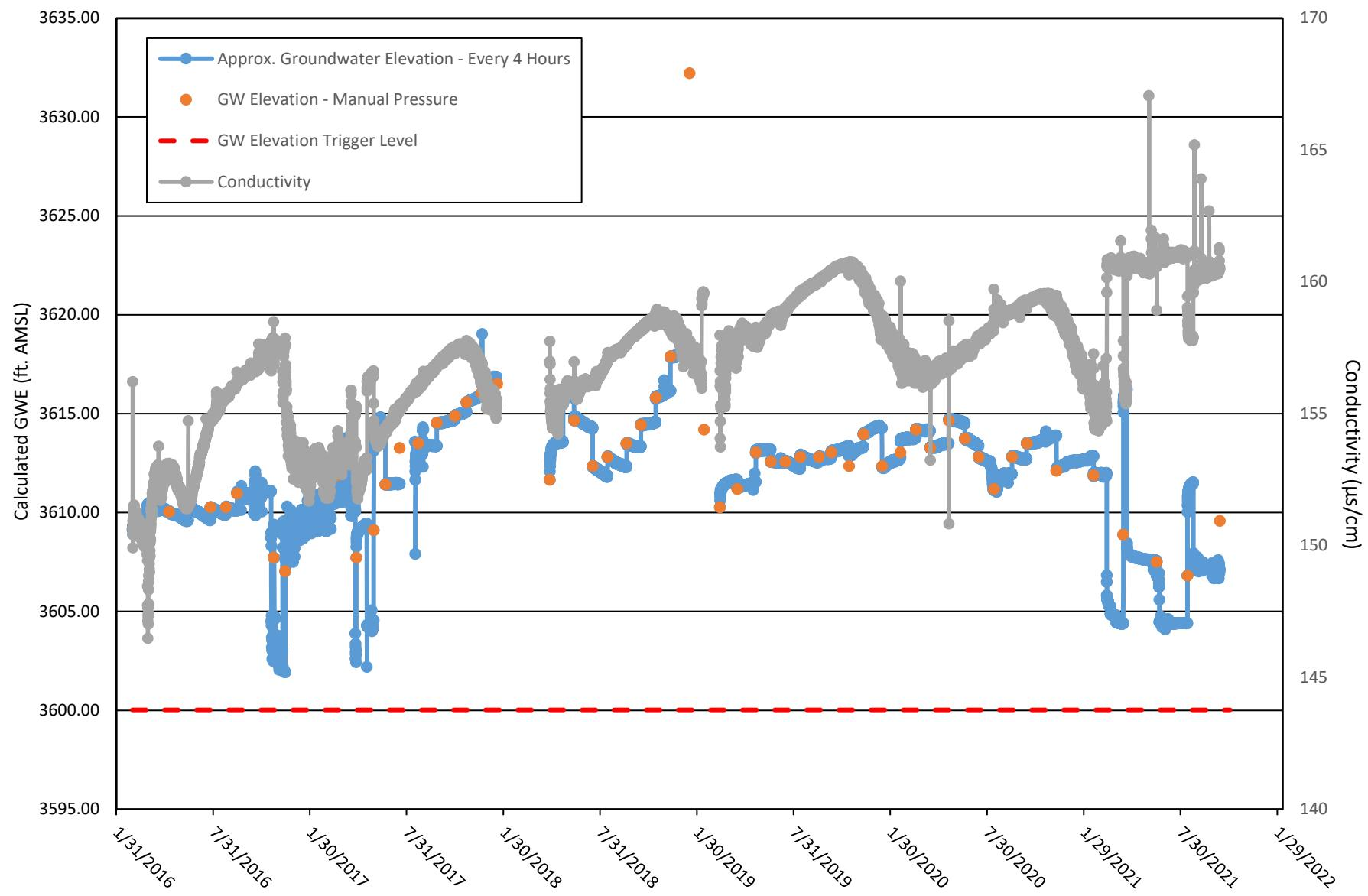
Note: Artesian Well. Transducer data from AquaTroll 200 correlated to reference pressure and converted to GWE.
