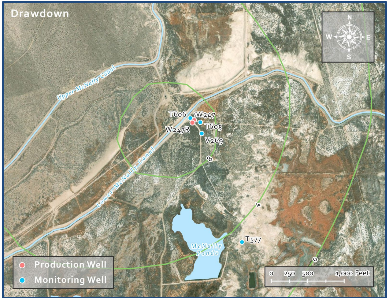
Figure 7 – Drawdown contours of groundwater levels in the shallow aquifer from pumping replacement well W247R at 5.3 cfs for one year
