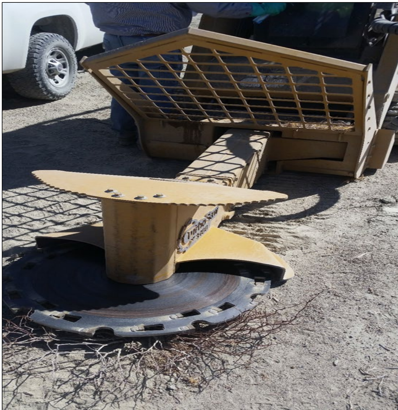
Saltcedar Figure 2. Turbosaw attachment used to cut larger diameter tamarisk trees and apply herbicide to the cut stumps
