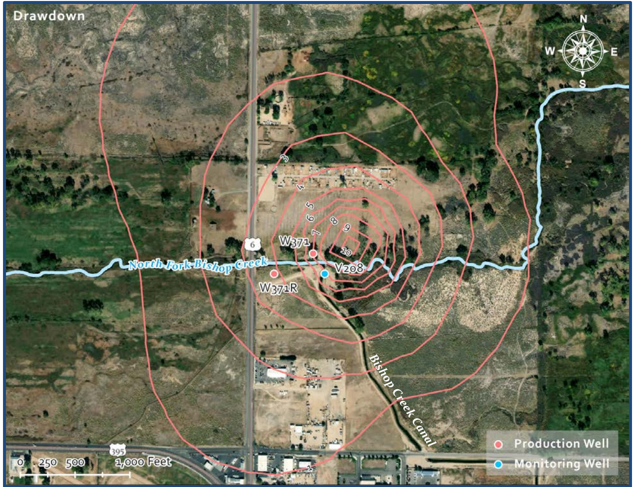
Figure 8 – Drawdown contours of groundwater levels in the shallow aquifer from pumping original W371 at 2.5 cfs for one year
