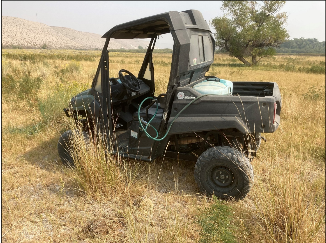
Weed Figure 3. Utility terrain vehicle with mounted herbicide spray system
