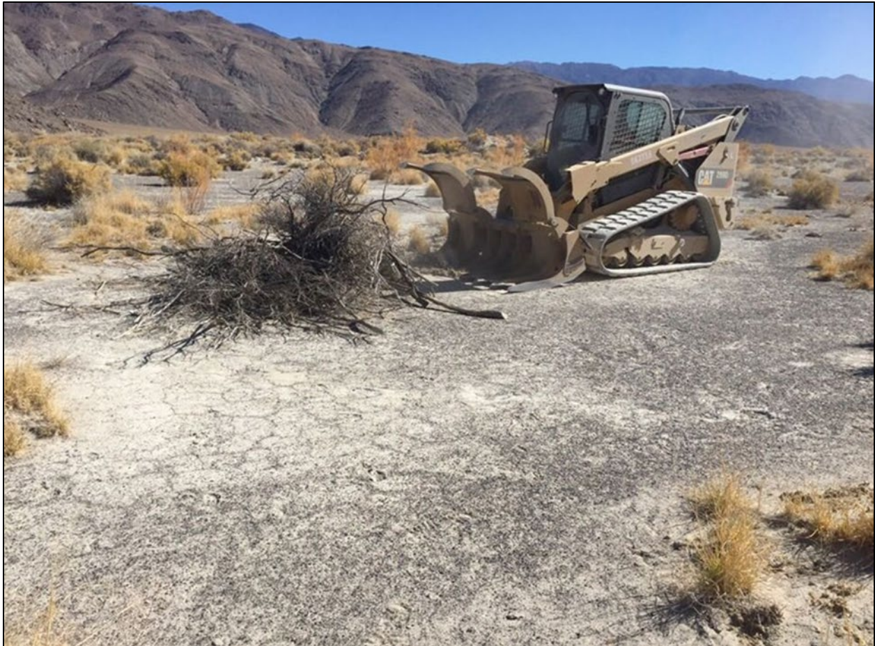
Saltcedar Figure 3. Grapple rake used to collect and consolidate tamarisk slash
