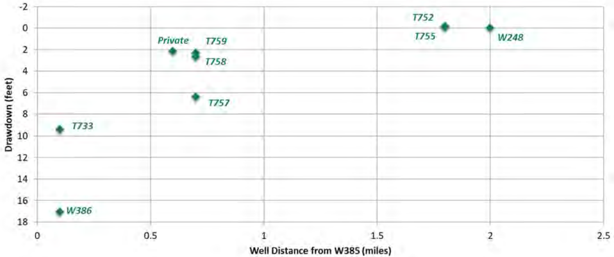
Figure 9 – Distance-Drawdown for Deep Wells End of W385 operational Test ( t = 64 days) with T759 and Private Well Added
