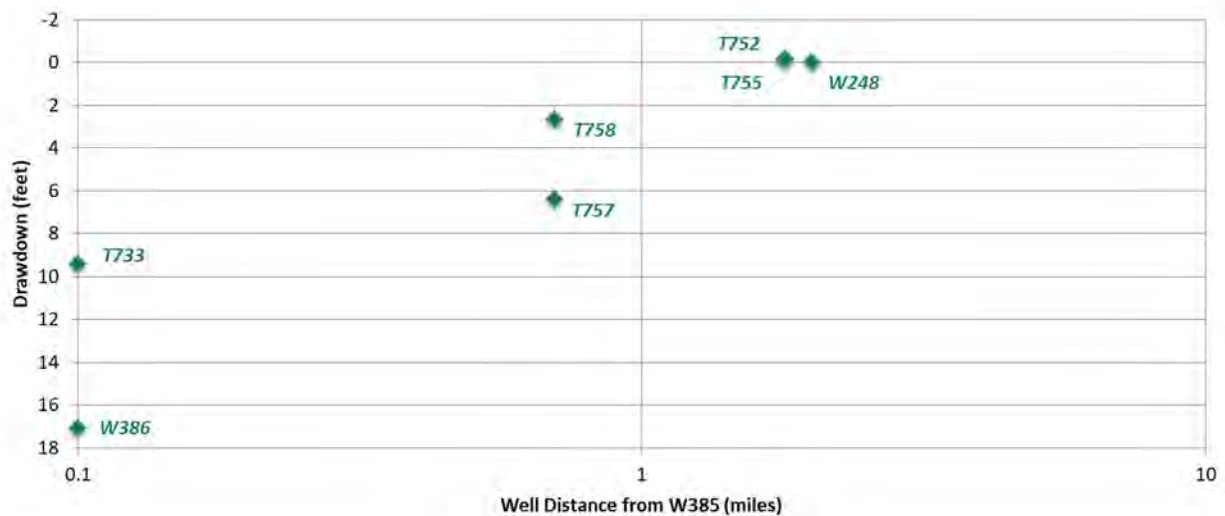
Figure 8 – Distance-Drawdown Plot for Deep Wells End of W385 operational Test ( t = 64 days) (Log x-axis)
