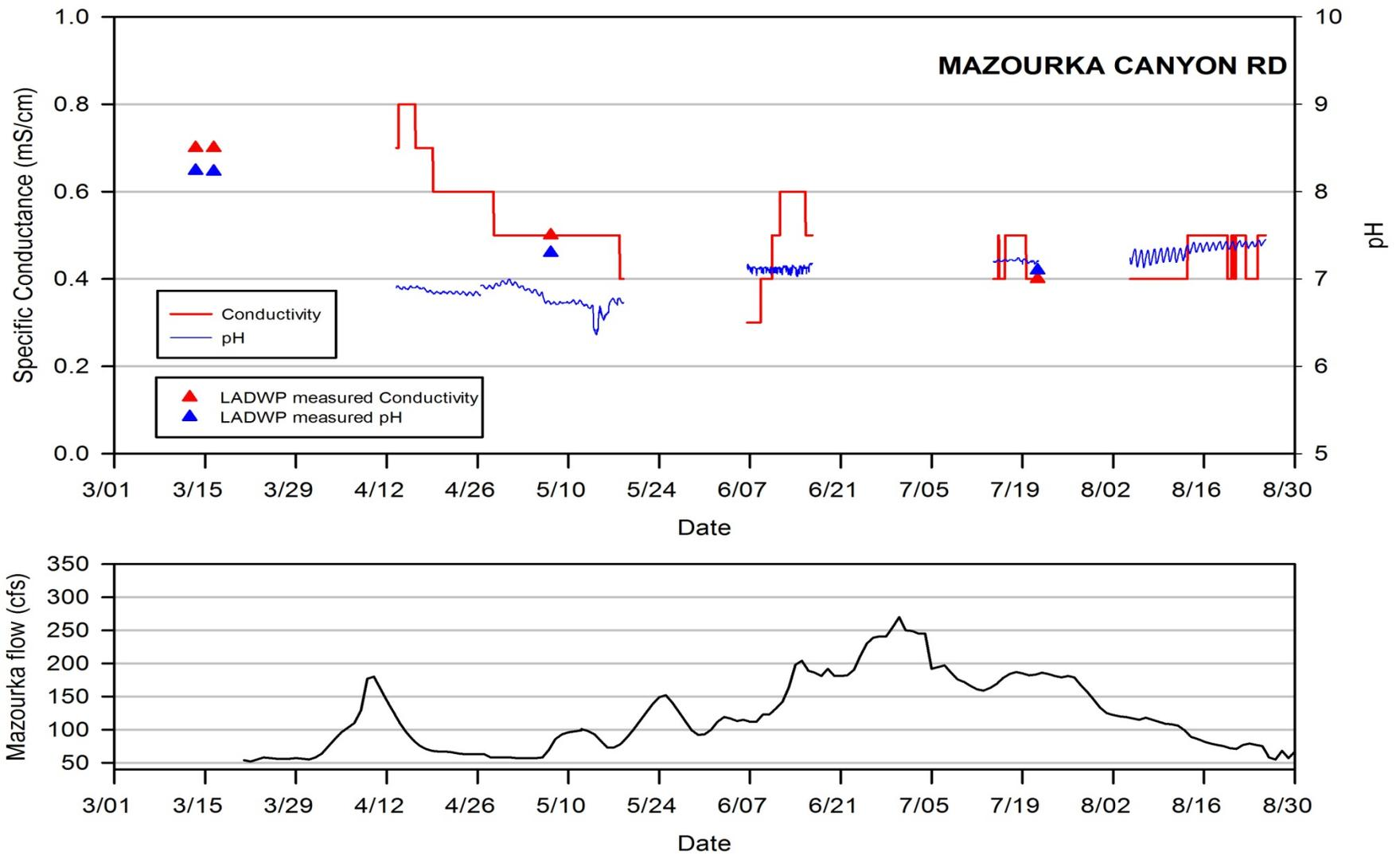
Figure 8. Specific Conductance and pH (top graph) and daily flow measured (bottom graph) at Mazourka Canyon Rd.
