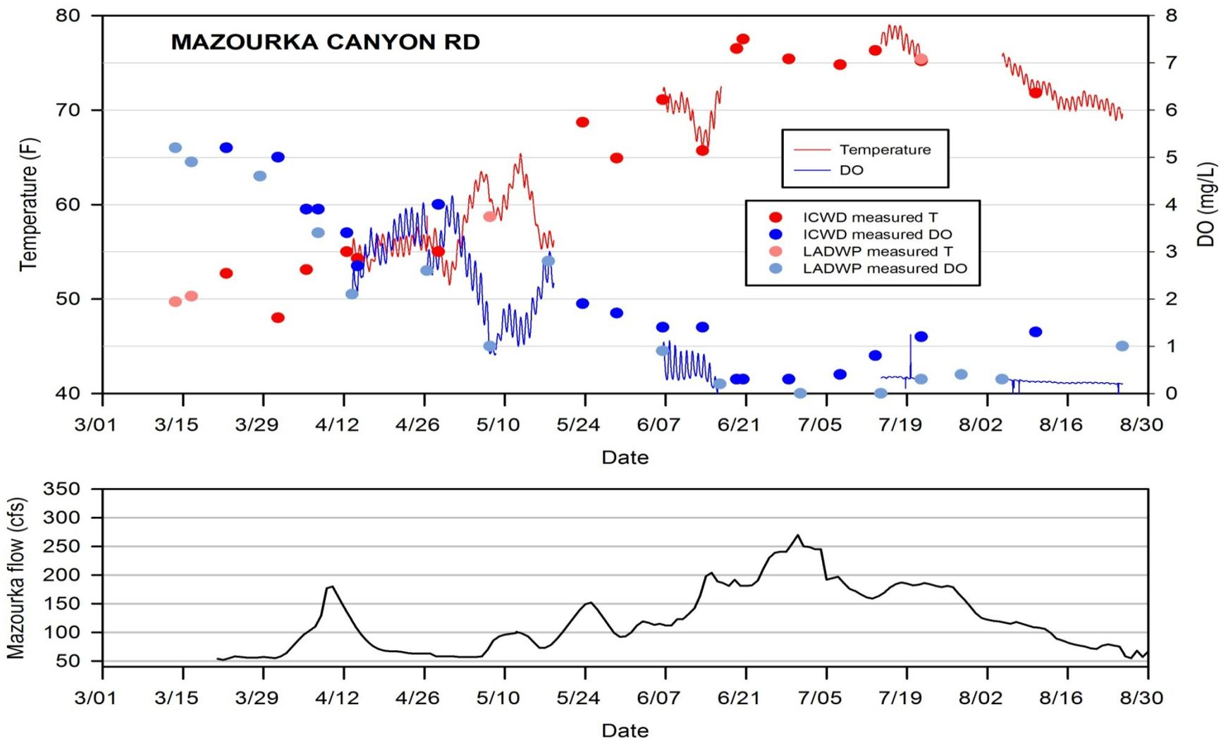
Figure 2. Dissolved oxygen and temperature (top graph) and daily flow (bottom graph) measured at Mazourka Canyon Rd. Individual points are manual reads.
