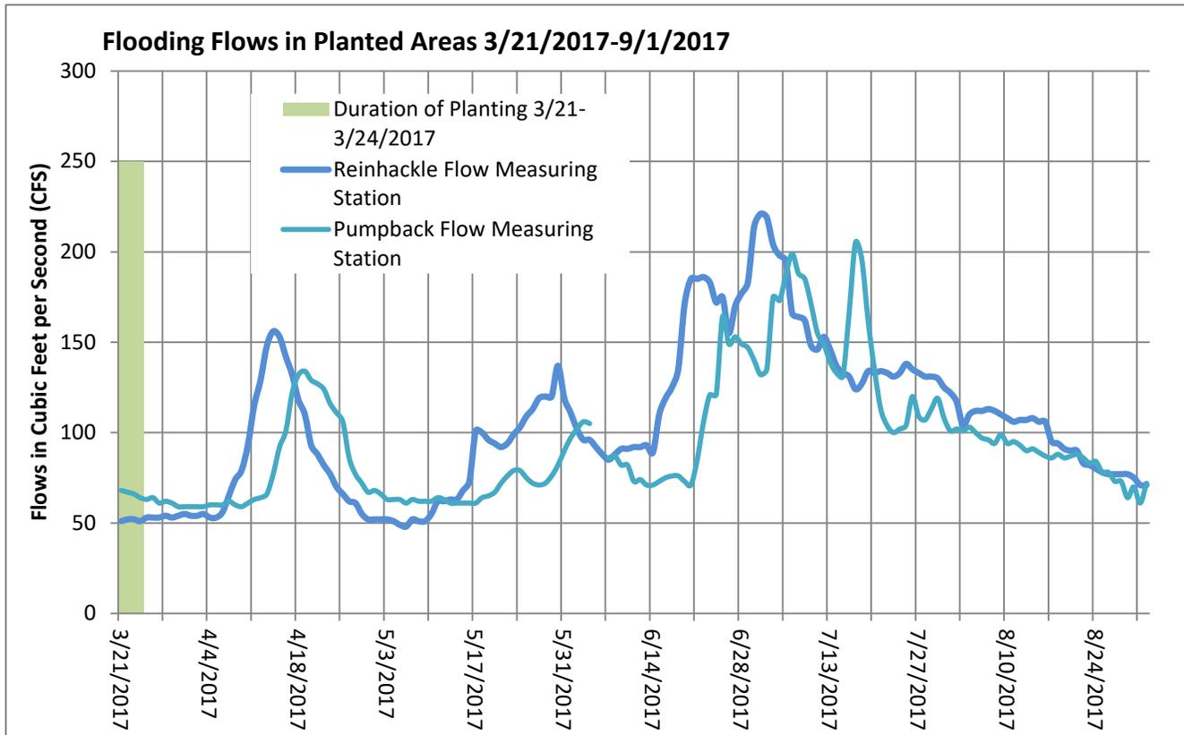
Figure 4. River flow above and below planting site. In a normal year the area would experience up to 90 cfs flow for a few days.
