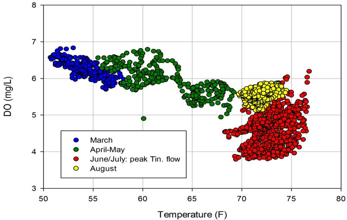
Figure 5. Intake DO as a function of temperature segregated by date showing the depressed DO during the peak Tinemaha releases in June and July.
