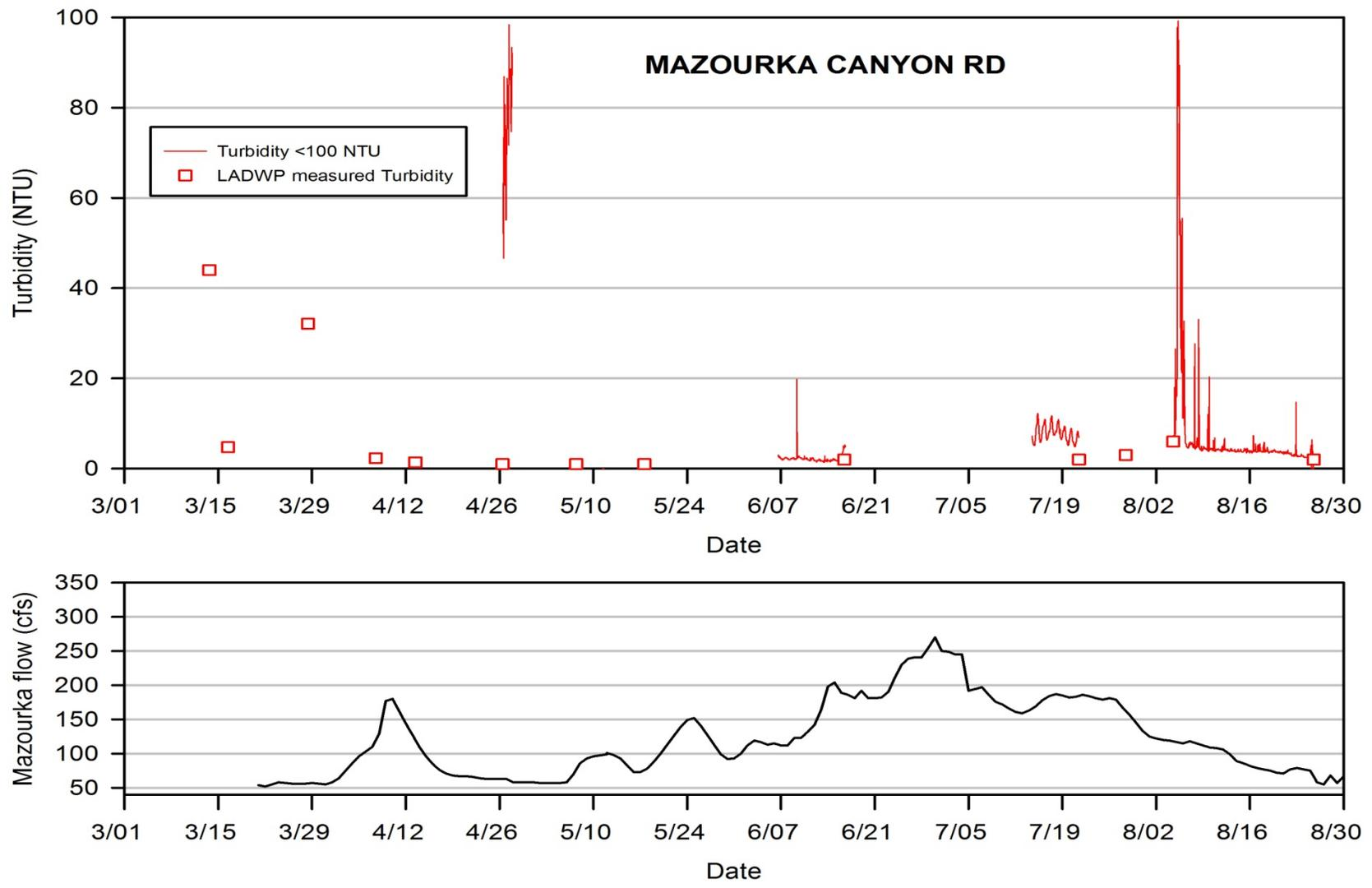
Figure 12. Turbidity (top graph) and daily flow measured (bottom graph) at Mazourka Canyon Rd.
