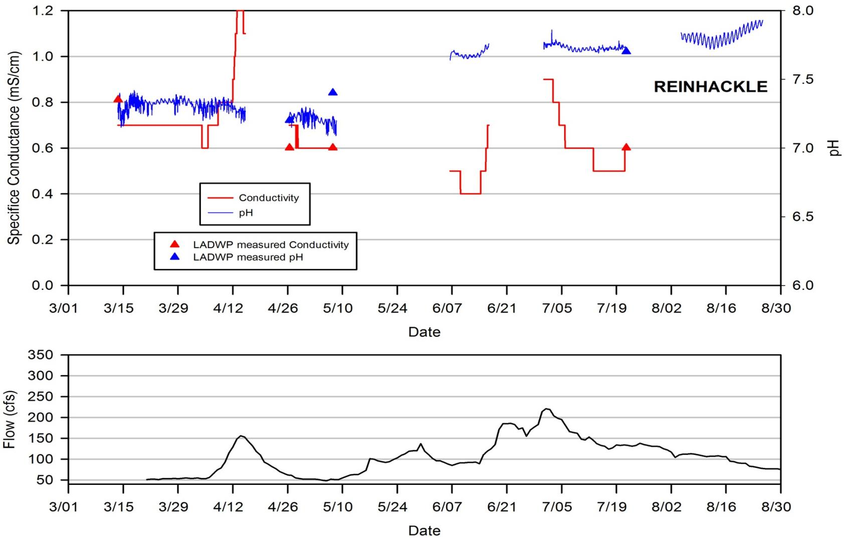
Figure 9. Specific Conductance and pH (top graph) and daily flow (bottom graph) measured at Reinhackle station.
