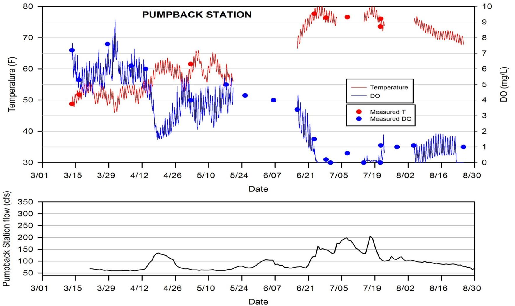
Figure 4. Dissolved oxygen and temperature (top graph) and estimated daily flow (bottom graph) arriving at the Pumpback Station. Individual points are manual reads.
