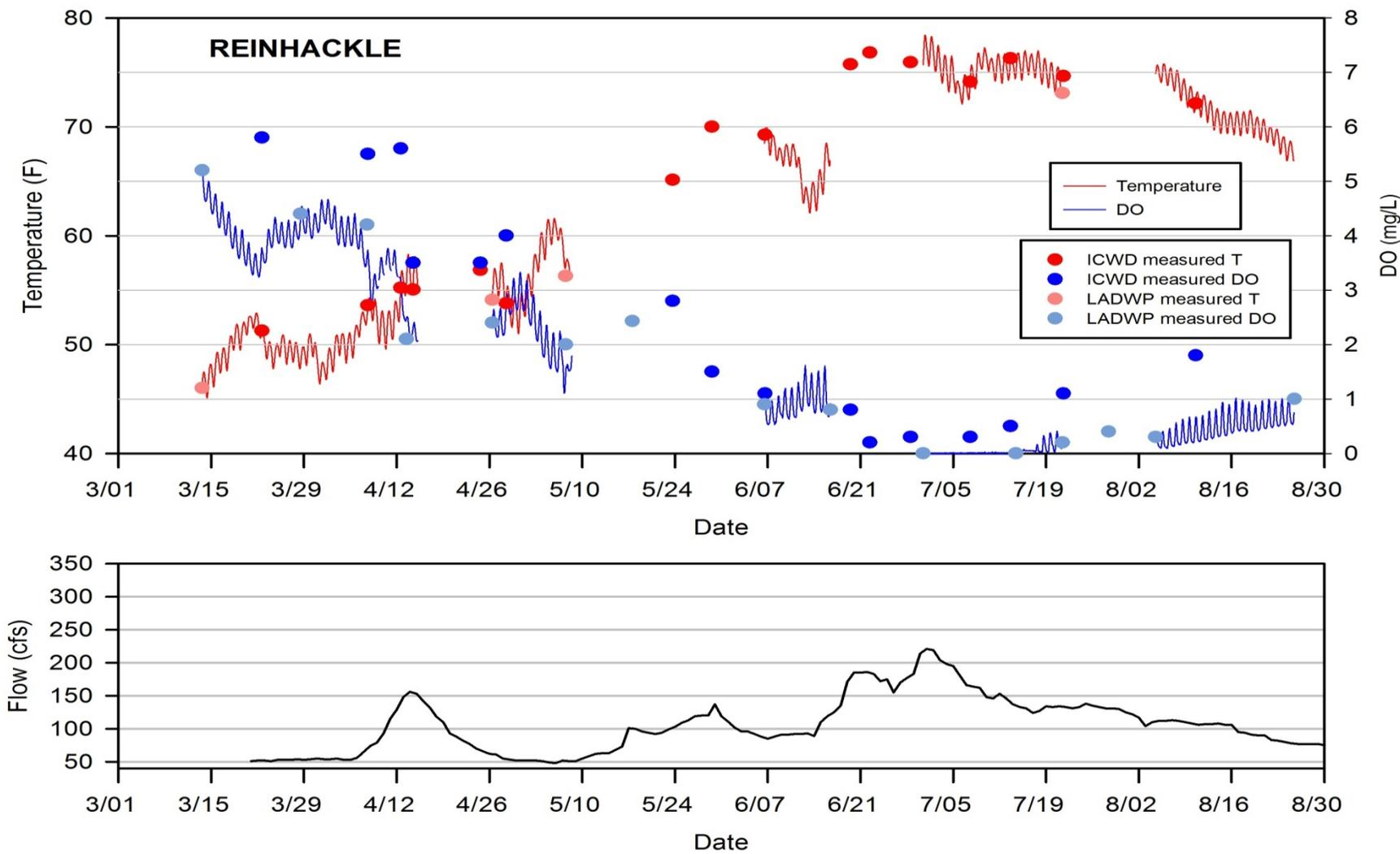
Figure 3. Dissolved oxygen and temperature (top graph) and daily flow (bottom graph) measured at Reinhackle station. Individual points are manual reads.
