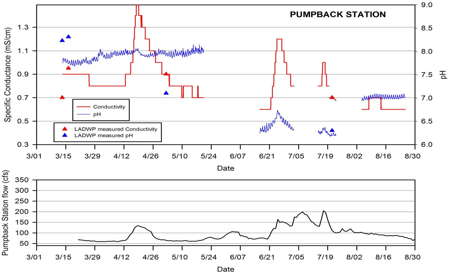
Figure 10. Specific Conductance and pH (top graph) and estimated daily flow (bottom graph) arriving at the Pumpback Station.
