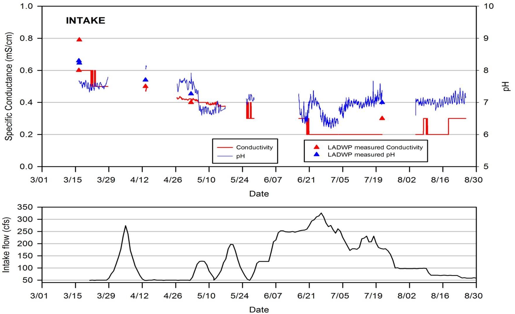
Figure 7. Specific Conductance and pH (top graph) and daily flow measured (bottom graph) at the Intake measuring station.
