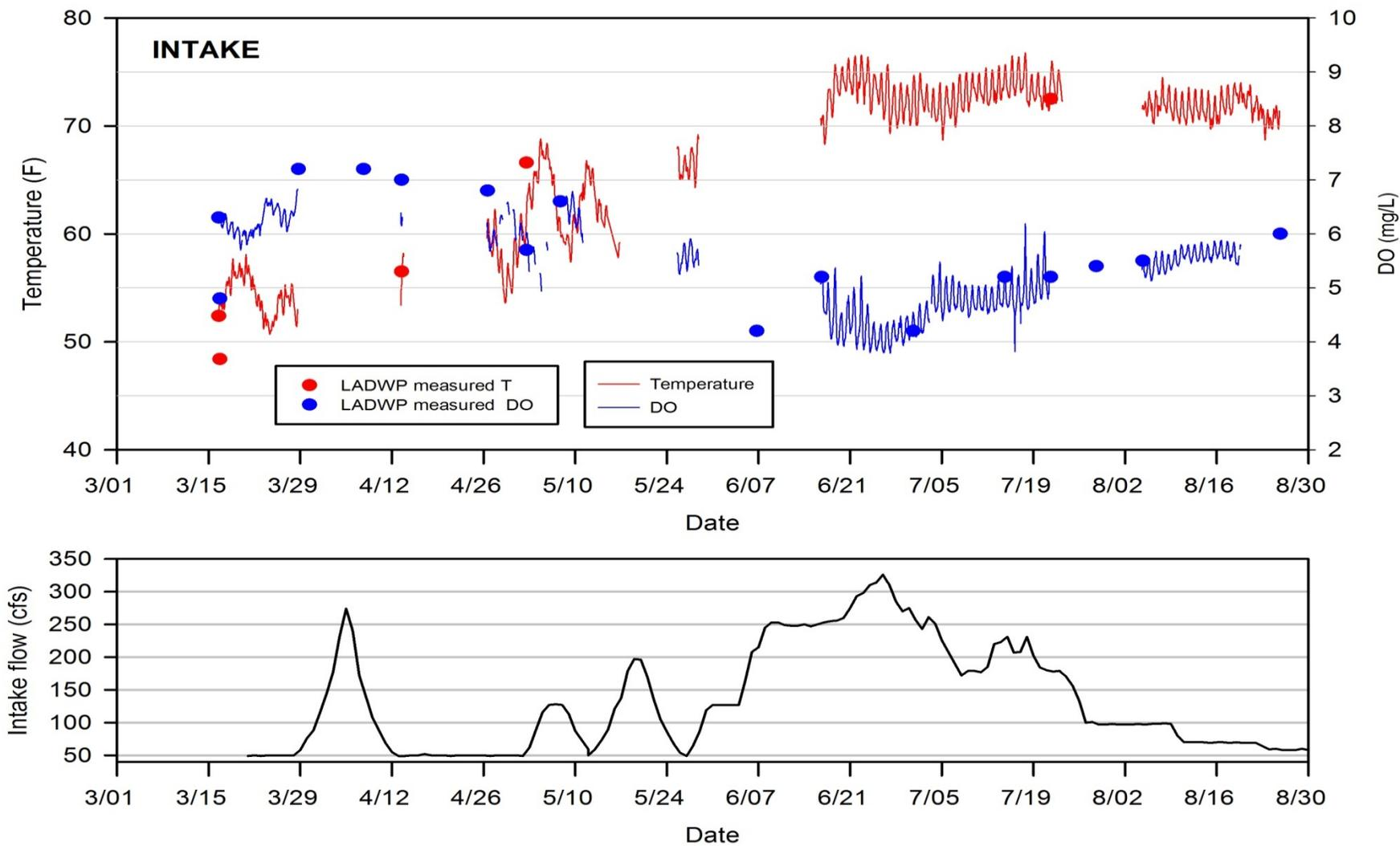
Figure 1. Dissolved oxygen and temperature (top graph) and daily flow (bottom graph) measured at the Intake measuring station. Individual points are manual reads.
