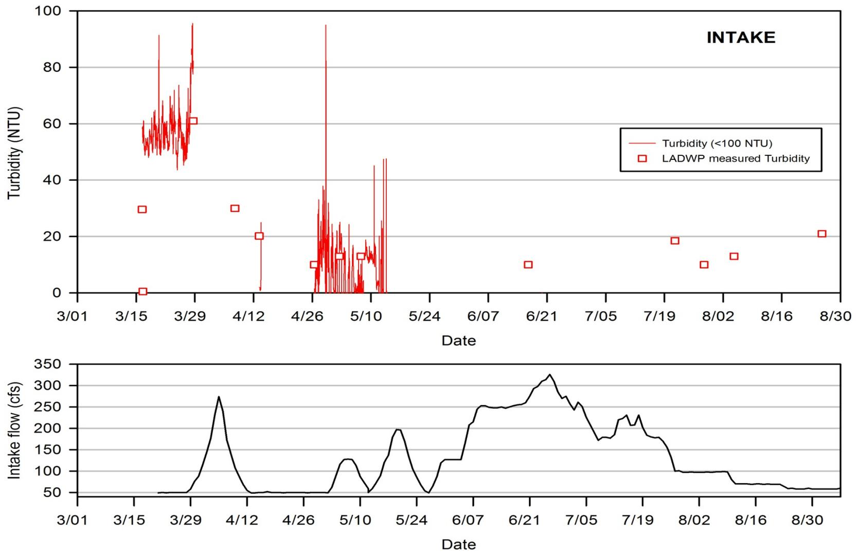
Figure 11. Turbidity (top graph) and daily flow measured (bottom graph) at the Intake measuring station.
