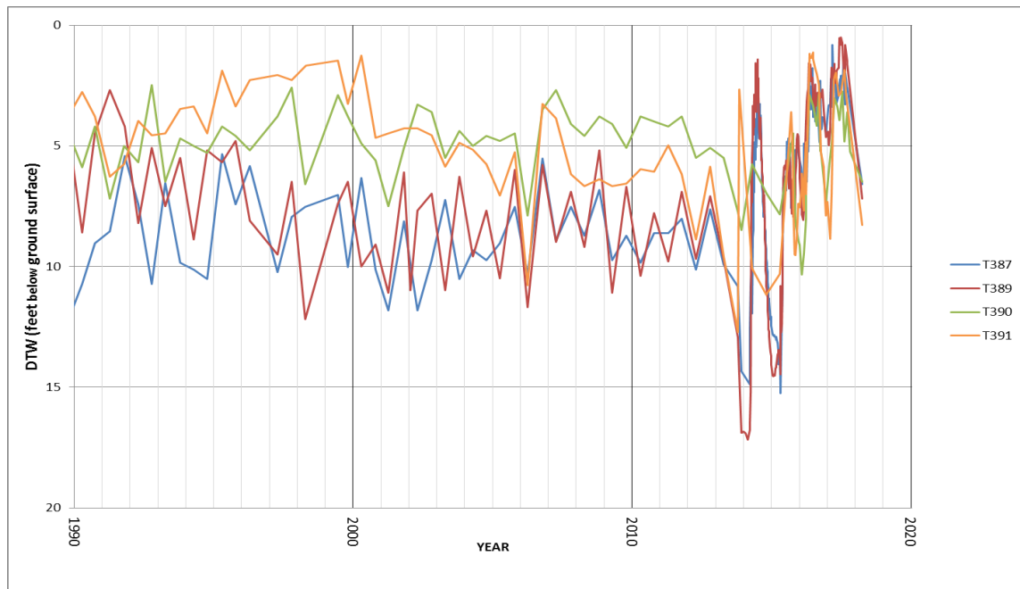
Figure 3.11.a. Hydrographs of selected monitoring wells in the western Bishop wellfield. Locations of the wells are shown in Figure 3.7
