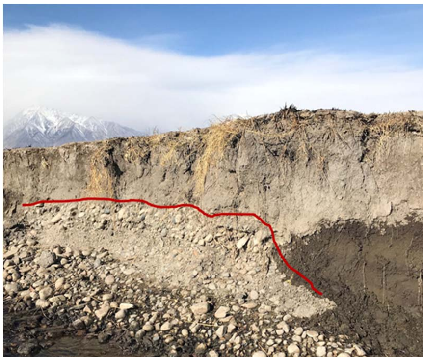
Figure 2. Exposure of finer textured soils over gravel-cobble layer in down-cut irrigation ditch in the Five Bridges Impact Area. The red line denotes the approximate boundary between the different parent materials. The extent of capillarity where fine-grained surface material intersects the shallow water table is apparent as the darker soil color on the right side of the photo.
