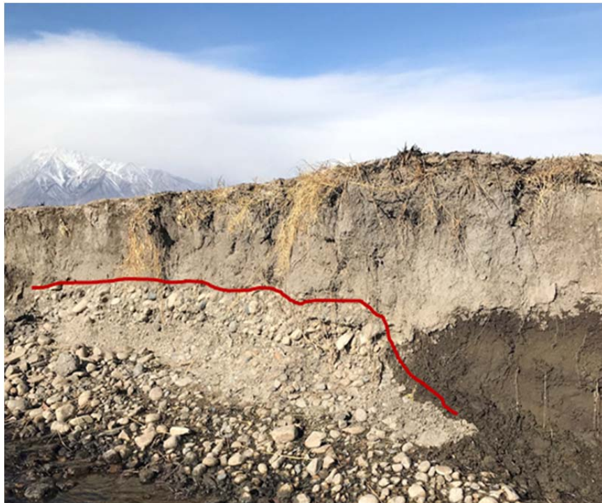
Figure 2. Exposure of finer textured soils over gravel-cobble layer in down-cut irrigation ditch in the Five Bridges Impact Area. The red line denotes the approximate boundary between the different parent materials. The extent of capillarity where fine-grained surface material intersects the shallow water table is apparent as the darker soil color on the right side of the photo.
