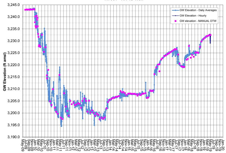
Note: Transducer data (absolute pressure) adjusted by data logged from BaroTroll and correlated to Manual DTW measurements. Screened interval 490-540 feet.
